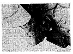
Fig. 8 1. Fuel lift pump 2. Manual priming lever
