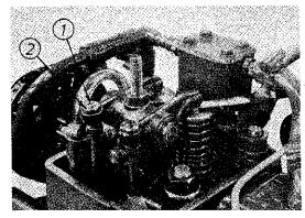
Fig. 14 1. Adjusting screw 2. Lock nut
