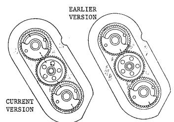
MARKS ON COUNTERWEIGHTS AND CRANK GEAR
