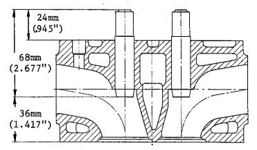
Dimensions for replacing valve guides
