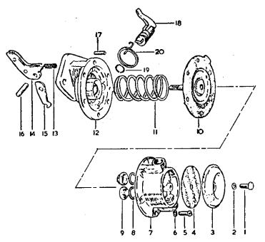
Reassembling is accomplished in reverse sequence. Notice that, when reassembling the valves, one valve must be turned with the flat side against the mark N. The other valve should be reassembled in the opposite direction.
