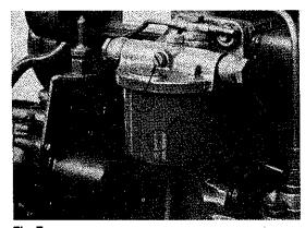
Fig. 7 1. Fuel filter 2. Slotted screw for bleeding
