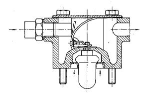
Fig. 22 Cross section of thermostat housing
