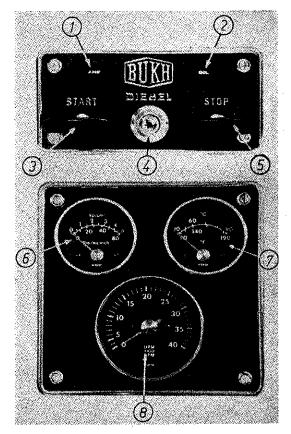
Fig. 9 Operating panel (standard) and instrument panel (additional)
