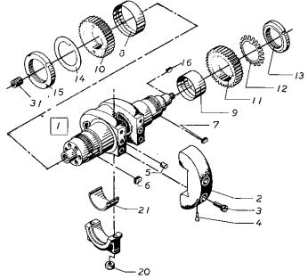
REAR MAIN AND INTERMEDIATE BEARINGS ENGINE SERIAL NO. BEARING YEAR Pilot 10 85000 & up 4400.1.E 1973 Pilot 20 92000 & up 4600.1.C 1973 When the crank shaft is removed per
