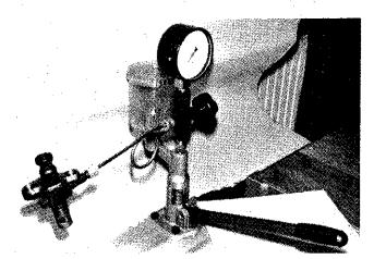
With the nozzle setting equipment (as shown above) it is possible to test: a) Opening pressure
