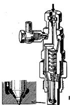
Fig. 18 Injection nozzle
