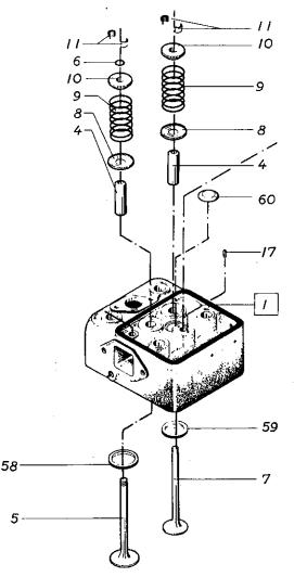
REPLACING VALVE GUIDES (Cont'd)
