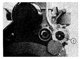
Fig. 20 1. Rubber rotor of cooling water pump
